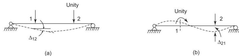
Fig. 6.15 | (a) Unit load at 2, (b) Unit moment at 1
