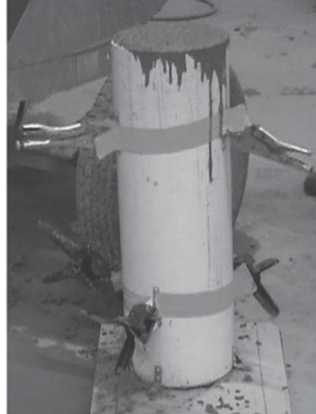
Fig. 7.7 Dimensions of column segregation apparatus
