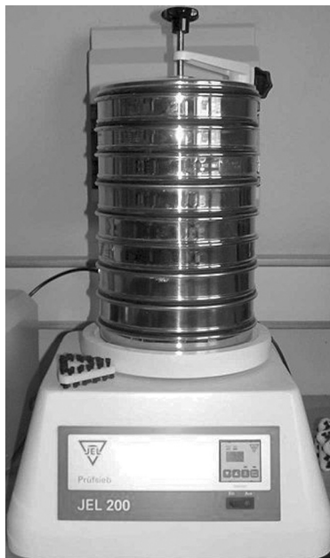
Fig. 4.12 Test sieves used for gradation of fine aggregate
