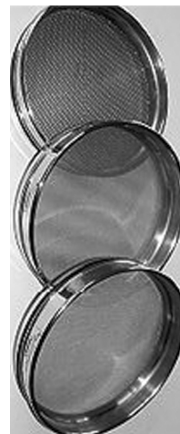
Fig. 4.12 Test sieves used for gradation of fine aggregate
