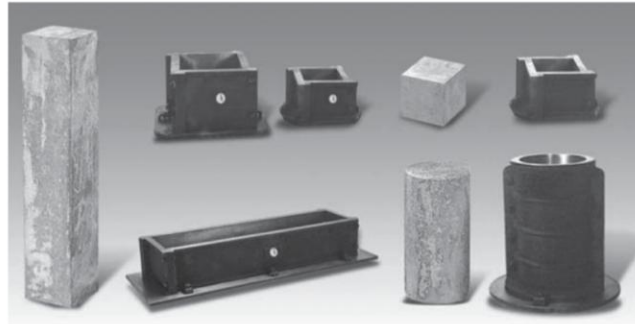
Fig. 8.4 Typical moulds and concrete specimens
