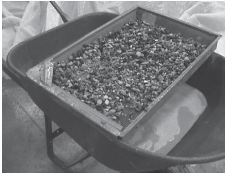
Fig. 7.8 Aggregate washed over No. 4 sieve from the column segregation apparatus
