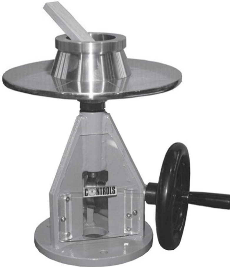
Fig. 3.6 Typical flow table, flow mould and tamper
