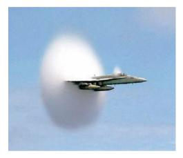
You are all familiar with sonic booms, those loud crashes of noise caused by aircraft flying faster than the speed of sound. You may have even heard a sonic boom, but you have probably never *seen* one. The remarkable photograph here shows water vapor outlining the surface of a shock wave created by an F-18 jet flying supersonically. (Note that there is also a small cone of water vapor trailing the back of the cockpit.)
