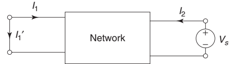
Fig. 9.38 Network for deriving condition for reciprocity
