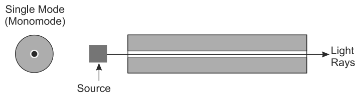
Fig. 10.18 Step-index fibre—single-mode operation
