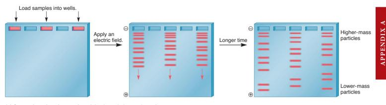
(a) Separation of a mixture of particles by gel electrophoresis
