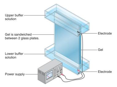
(b) Apparatus used in gel electrophoresis
