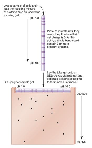
(a) The technique of two-dimensional gel electrophoresis
