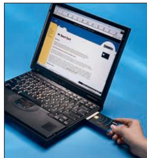
Figure 4-20 Inserting a PC card into a notebook computer
