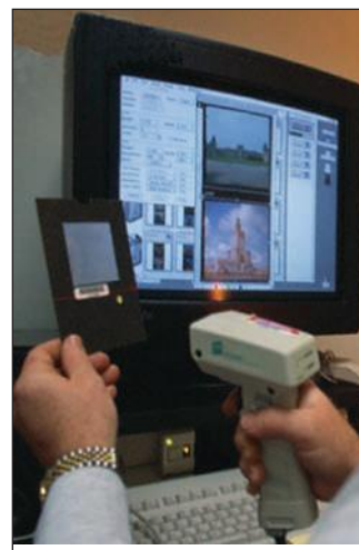
Figure 2-15 A wand reader is used to record product codes
