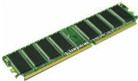
Figure 4-14 RAM chips mounted on circuit board
