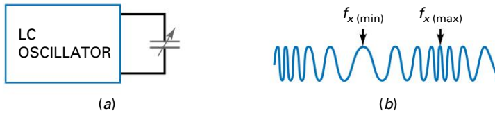
Figure 23-48 (a) Variable capacitance changes resonant frequency of LC oscillator; (b) sine wave has been frequency-modulated.
