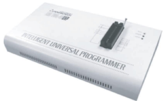
Fig. 12.1 Firmware Embedding Tool-Device Programmer: LabTool-48UXP)
