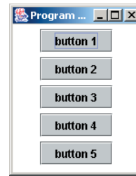
Figure 14.12 Placement of five buttons by using FlowLayout when the frame is first opened and after the frame is resized.
