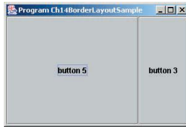
Figure 14.14 Placement of two buttons by using BorderLayout . Buttons are placed on the center and east regions.
