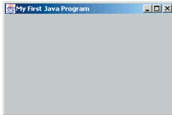
Figure 2.1 Result of running the Ch2Sample1 program. The window size is 300 by 200 pixels and has the title My First Java Program .
