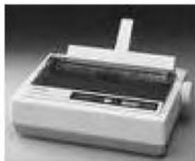
Figure 3.7 : Dot Matrix Printer
