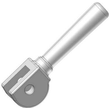
Fig. 15.33 A cam clamp used for quick and easy clamping a part
