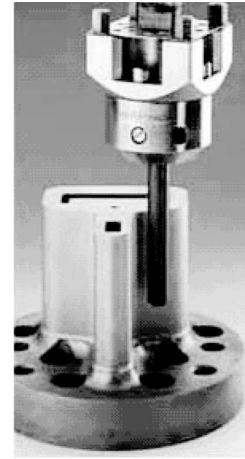
Fig. 11.22 Typical example of EDM milling producing a complex work piece with simple cylindrical electrode
