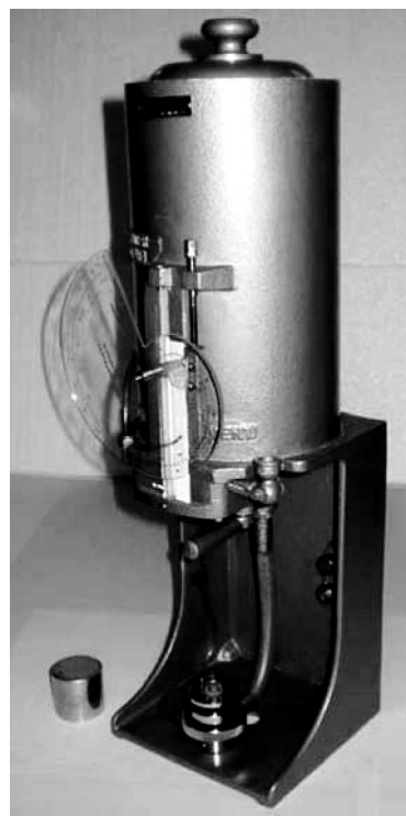
FIG. 3.22 Permeability meter for measuring the permeability of green sand
