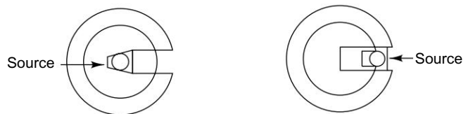
Fig. 2.16 Gamma Ray Camera with Source Rotating Mechanism
