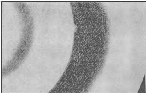
Oxide inclusions in Mg-Zn-Zr alloy casting
