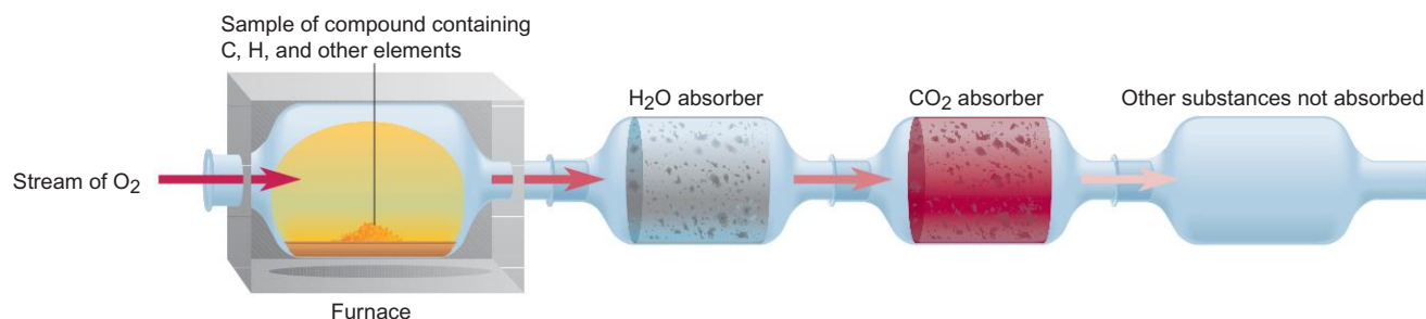
Figure 3.5 Combustion apparatus for determining formulas of organic compounds. A sample of compound that contains C and H (and perhaps other elements) is burned in a stream of O 2 gas. The CO 2 and H 2 O formed are absorbed separately, while any other element
