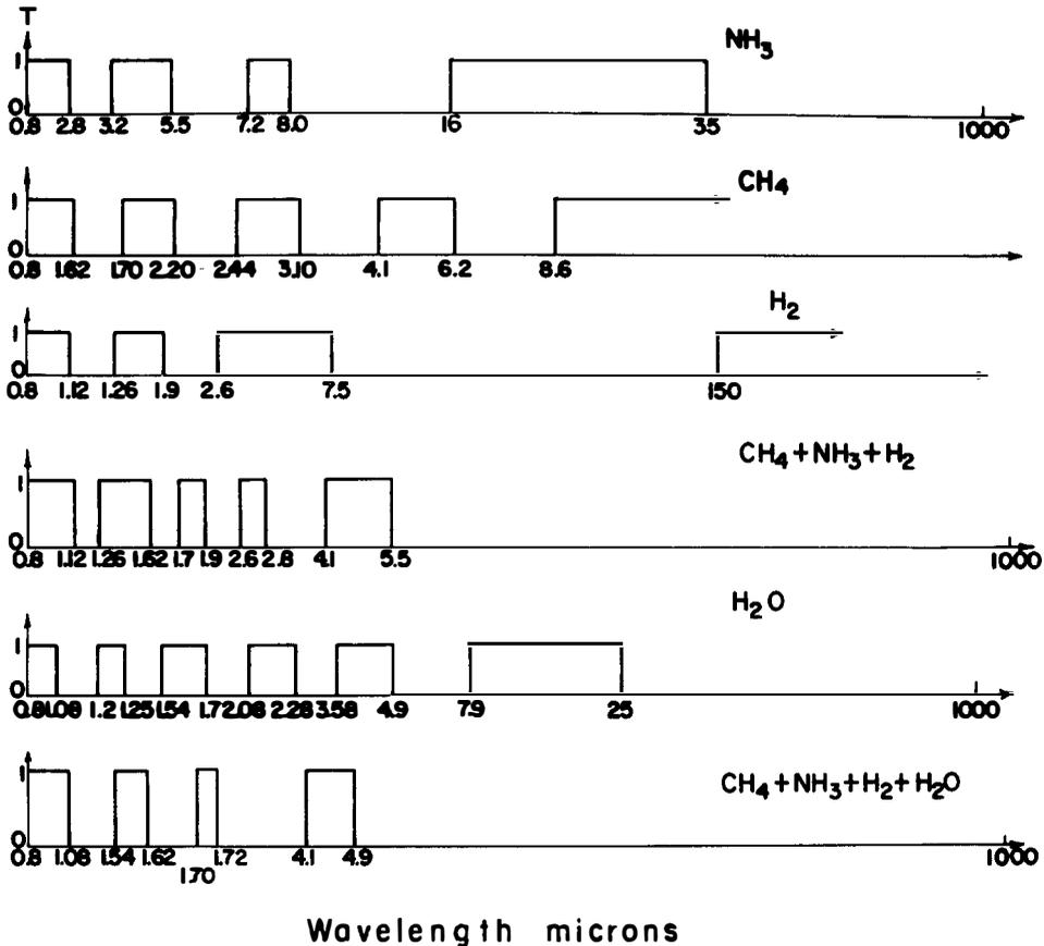
FIG. 1. Step function approximation to the transmission spectra of  $\text{CH}_4$ ,  $\text{NH}_3$ ,  $\text{H}_2\text{O}$ , and  $\text{H}_2$ , based on laboratory spectra (courtesy of Dr. B. N. Khare) and theoretical calculations (courtesy of Dr. L. D. G. Young) for paths and pressure broadening appropriate for Jupiter. Various combined spectra are also shown.  $T$  is the transmissivity.
