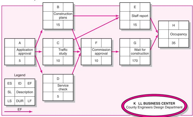
FIGURE 6.6 Activity-on-Node Network Forward Pass
