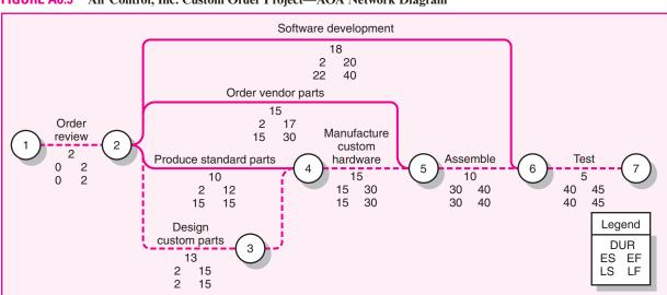
FIGURE A6.9 Air Control, Inc. Custom Order Project—AOA Network Diagram
