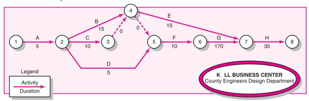
FIGURE A6.6 Activity-on-Arrow Network Forward Pass
