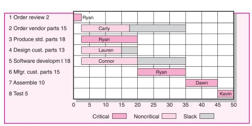
FIGURE A8.3 Air Control Project: CCPM Network
