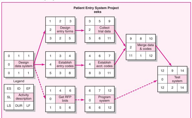
**FIGURE 8.16 Patient Entry Time-Phased Work Packages Assigned**
