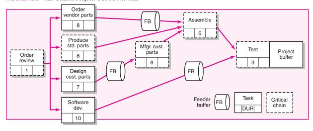
FIGURE A8.4 Air Control Project Gantt Chart: CCPM Network
