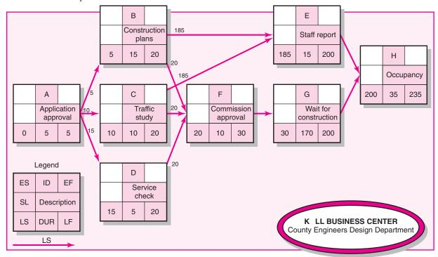
FIGURE 6.7 Activity-on-Node Network Backward Pass
